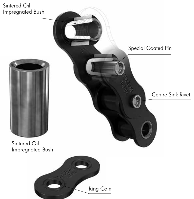
Fig. 10 Basic Construction
